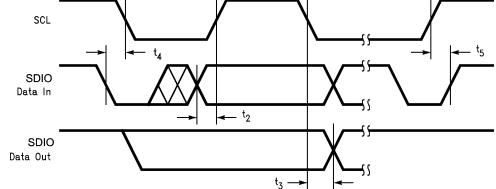
Figure 4. I<sup>2</sup>C Timing Diagram
