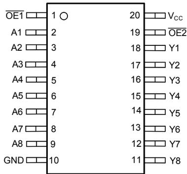
**Figure 4-1. PW and DGS Package,
