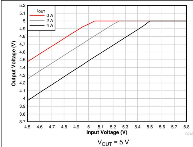
Figure 7-9. Voltage Dropout
