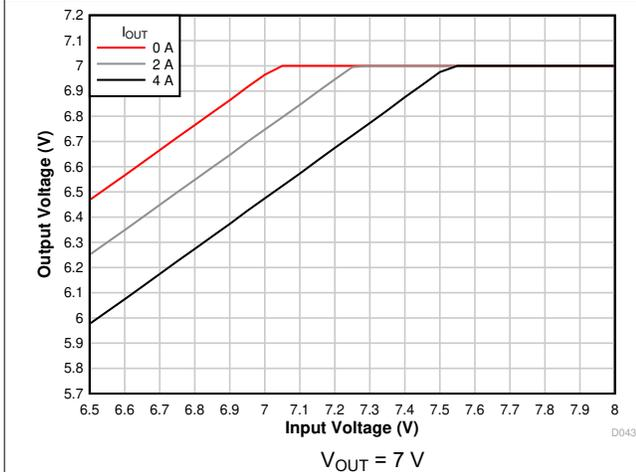
Figure 7-11. Voltage Dropout
