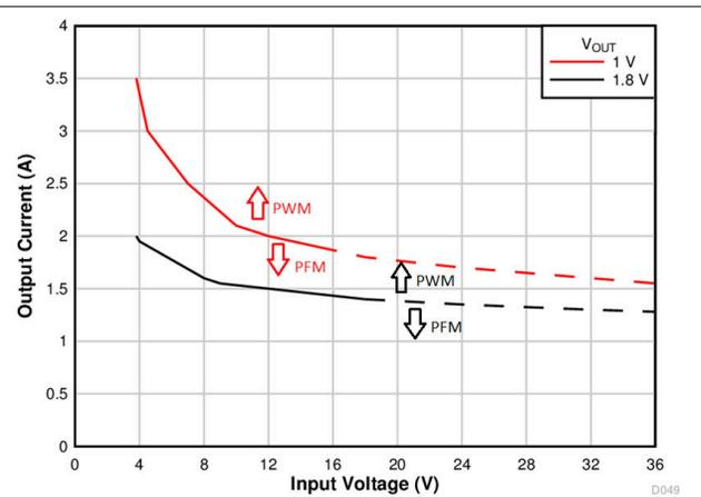
Figure 7-15. PFM/PWM Thresholds (1 V and 1.8 V)
