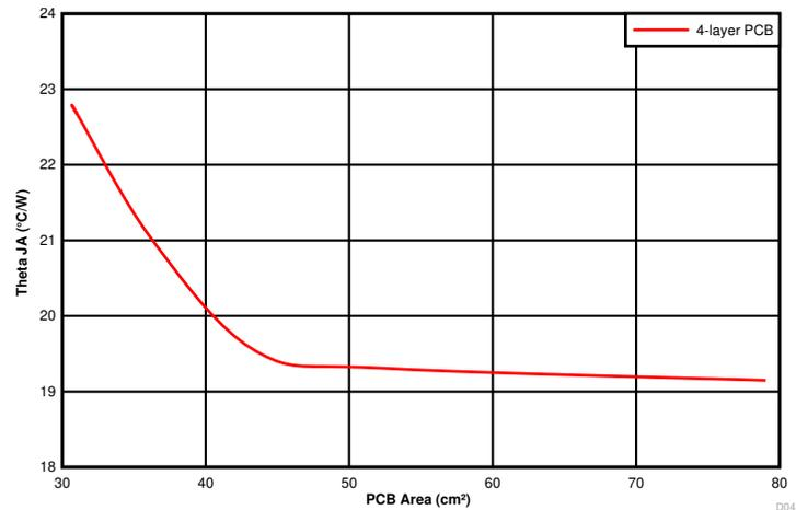
**Figure 10-4.  $R_{\theta JA}$  versus PCB Area (per Layer)**
