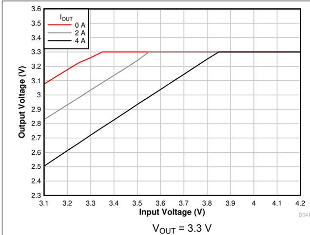
Figure 7-7. Voltage Dropout
