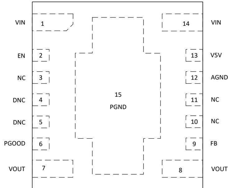
**Figure 5-1. 15-Pin QFN RDA Package (Top View)**
