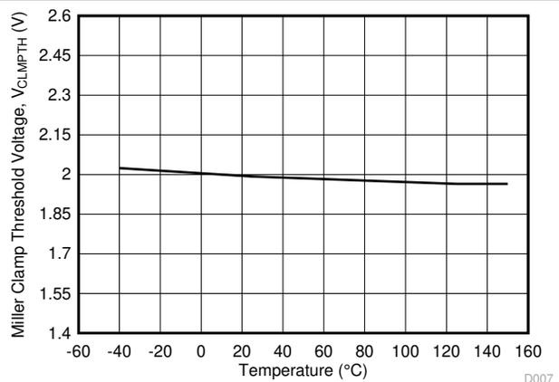
Figure 5-20.  $V_{CLMPH}$  Miller Clamp Threshold Voltage vs Temperature
