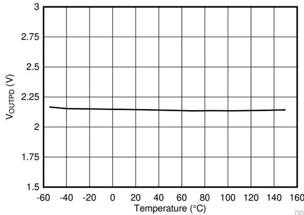
Figure 5-17.  $V_{OUTPD}$  Output Active Pulldown Voltage vs Temperature
