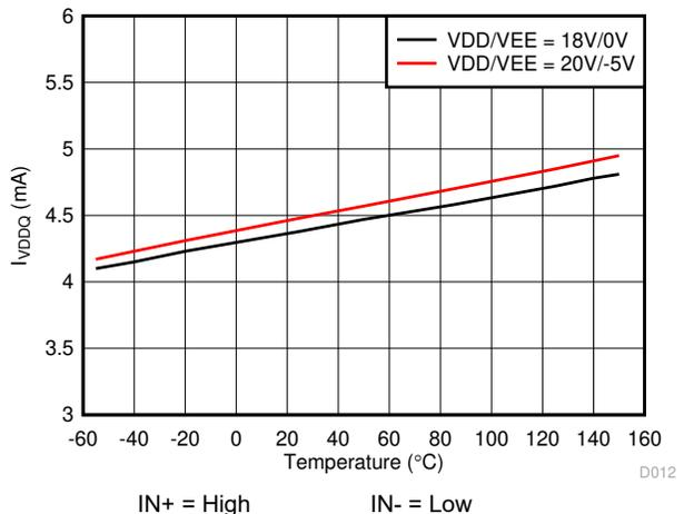
Figure 5-8. I<sub>VDDQ</sub> Supply Current vs Temperature
