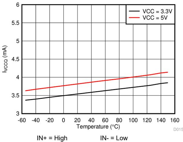
Figure 5-5. I<sub>VCCQ</sub> Supply Current vs Temperature
