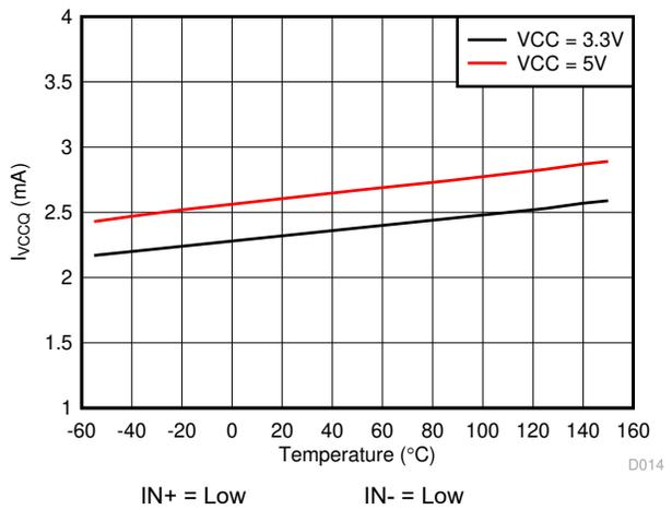
Figure 5-6. I<sub>VCCQ</sub> Supply Current vs Temperature
