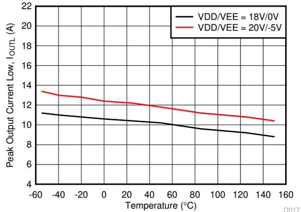
Figure 5-4. Output Low Driver Current vs Temperature
