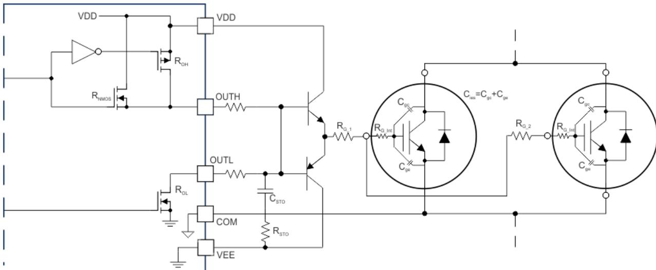
Figure 8-13. Current Buffer for Increased Drive Strength
