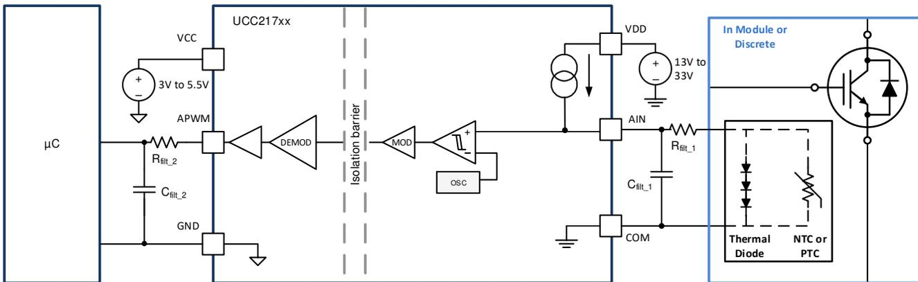
Figure 8-8. APWM Channel with Filtered Output
