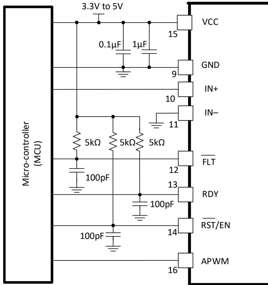
Figure 8-3.  $\overline{\text{FLT}}$ , RDY and  $\overline{\text{RST/EN}}$  Pins Circuitry
