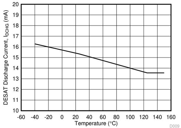
Figure 5-29.  $I_{\text{DCHG}}$  DESAT Discharge Current vs Temperature
