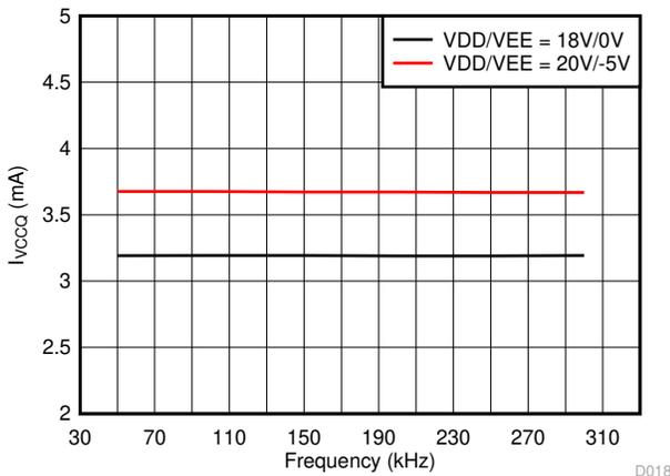
Figure 5-7. I<sub>VCCQ</sub> Supply Current vs Input Frequency
