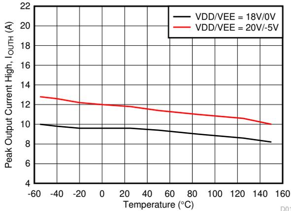
Figure 5-3. Output High Drive Current vs Temperature
