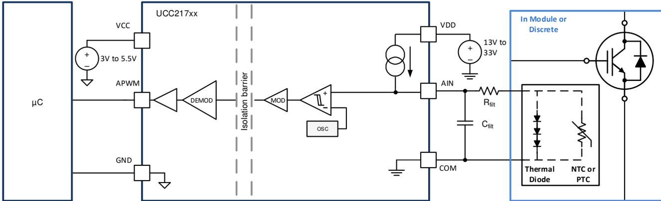
Figure 8-7. Thermal Diode or Thermistor Temperature Sensing Configuration
