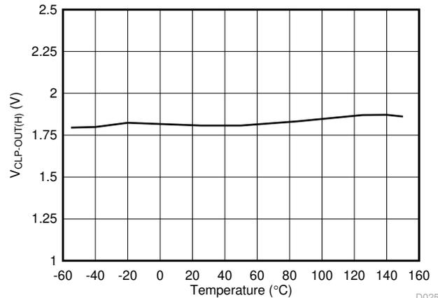
Figure 5-18.  $V_{CLP-OUT(H)}$  Short Circuit Clamping Voltage vs Temperature
