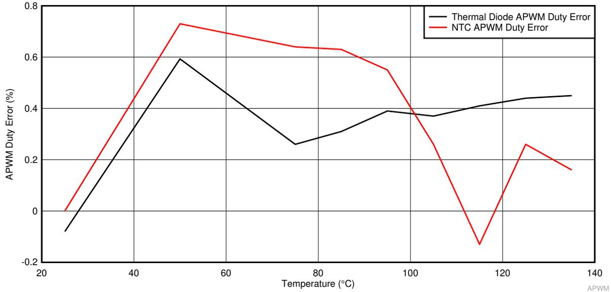
Figure 8-11. APWM Duty Error with Single-Point Calibration
