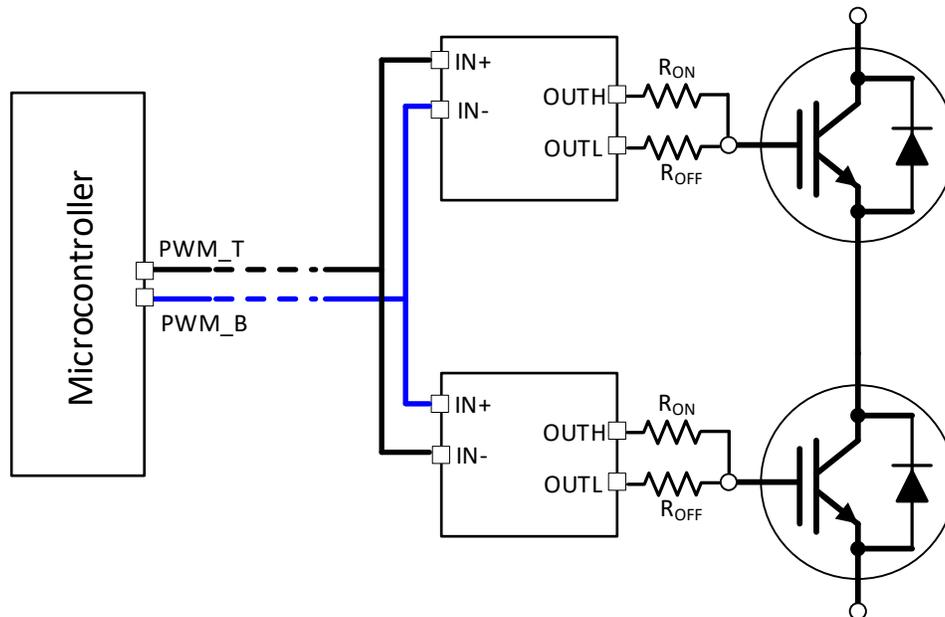
Figure 8-2. PWM Interlock for a Half Bridge
