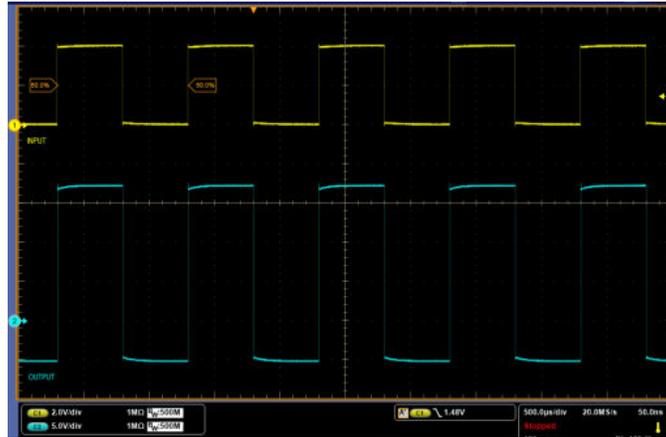
Figure 8-14. PWM Input (yellow) and Driver Output (blue)
