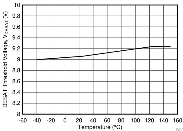
Figure 5-23.  $V_{DESAT}$  DESAT Threshold Voltage vs Temperature
