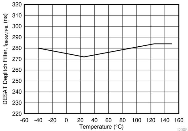
Figure 5-27.  $t_{\text{DESATFIL}}$  DESAT Deglitch Filter vs Temperature
