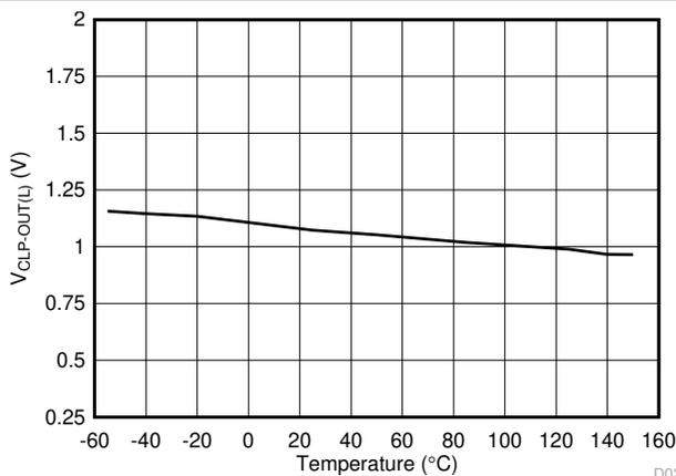
Figure 5-19.  $V_{CLP-OUT(L)}$  Short Circuit Clamping Voltage vs Temperature
