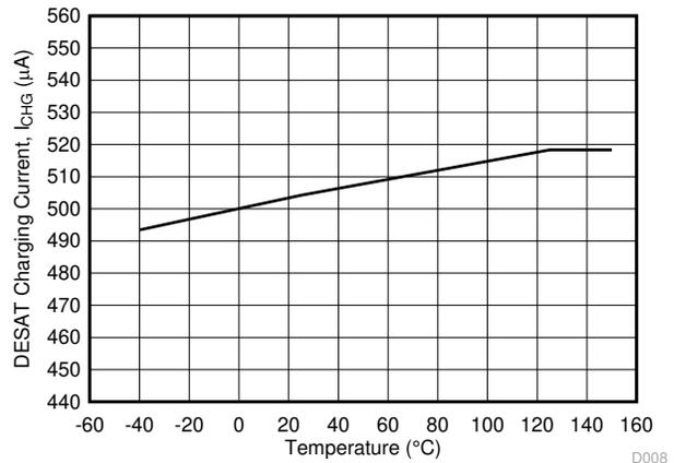
Figure 5-28.  $I_{\text{CHG}}$  DESAT Charging Current vs Temperature
