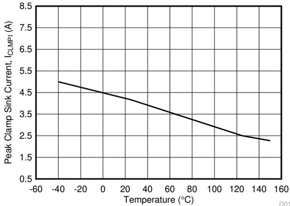
Figure 5-21.  $I_{CLMPL}$  Miller Clamp Sink Current vs Temperature
