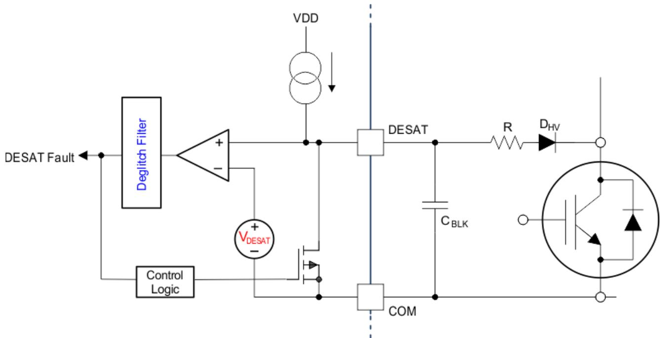
**Figure 7-5. DESAT Protection**
