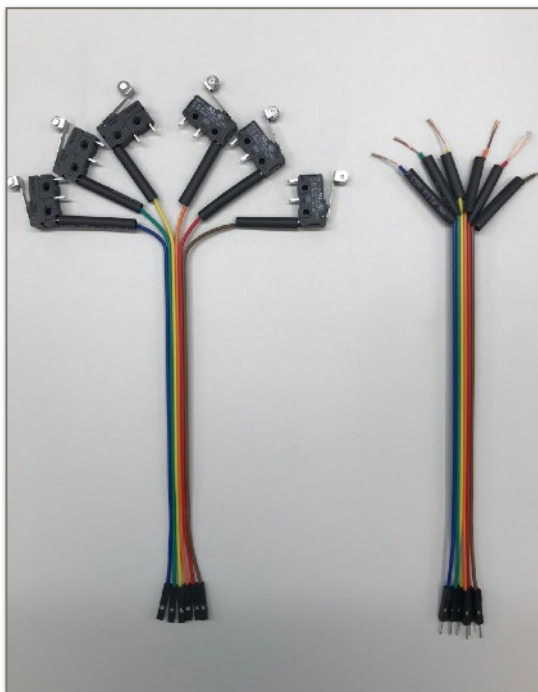
Slide a heat shrink tube (a) on each wire.
