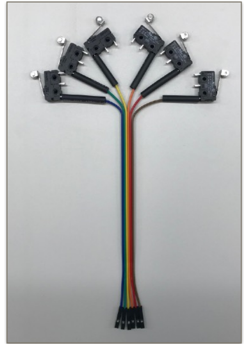
Solder one female wire on the "1" or "C" connection on each bump switch (0).
