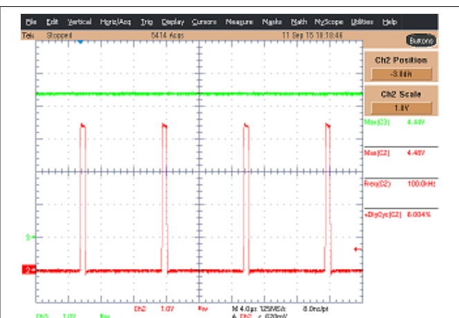
Figure 8-9. Supply Voltage 5 V Peak Signal 4.5 V
