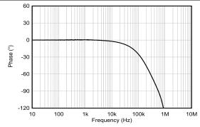
Figure 6-12. Phase vs Frequency, All Gains
