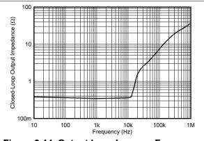
Figure 6-14. Output Impedance vs Frequency
