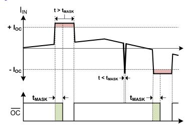
Figure 8-9. Overcurrent Detection MASK Diagram
