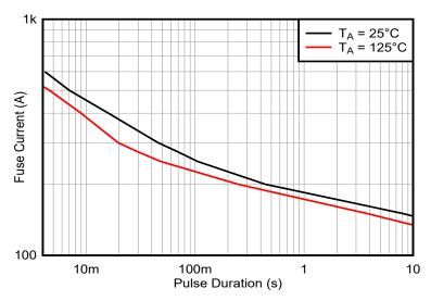
Figure 7-9. Single-Pulse Leadframe Capability
