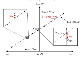
Figure 7-1. Sensitivity, Offset, and Nonlinearity Error
