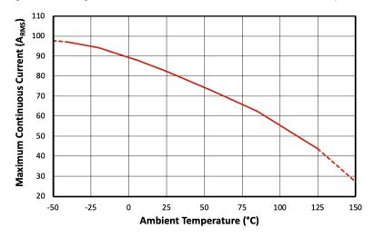
Figure 7-4. Maximum Continuous RMS Current vs Ambient Temperature
