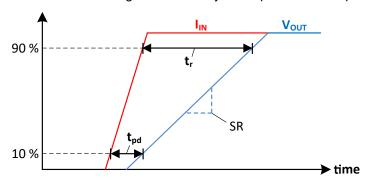
Figure 7-2. Transient Step Response
