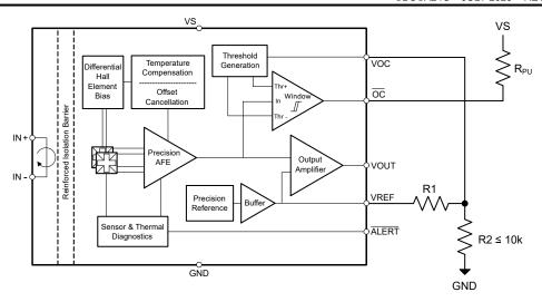
Figure 8-7. User Configurable Overcurrent Threshold Using Zero Current Output Reference Voltage
