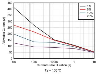
Figure 7-7. Maximum Repetitive Pulsed Current vs. Pulse Duration
