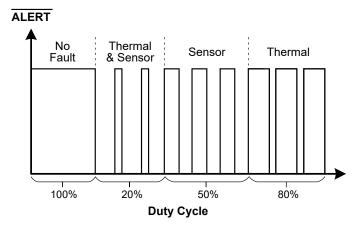
Figure 8-10. Sensor Diagnostics Waveform
