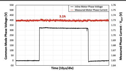
Figure 9-3. Inline Motor Current-Sense Input and Output Signals
