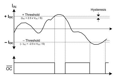
Figure 8-8. Overcurrent Output Response
