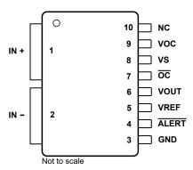
Figure 5-1. DVG Package 10-Pin SOIC Top View
