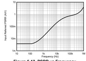
Figure 6-13. PSRR vs Frequency
