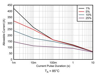
Figure 7-6. Maximum Repetitive Pulsed Current vs. Pulse Duration
