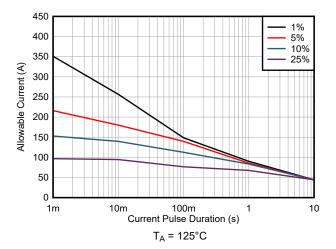
Figure 7-8. Maximum Repetitive Pulsed Current vs. Pulse Duration
