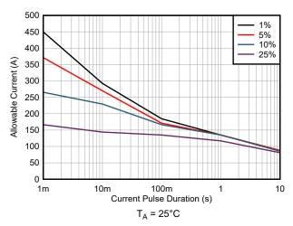
Figure 7-5. Maximum Repetitive Pulsed Current vs. Pulse Duration
