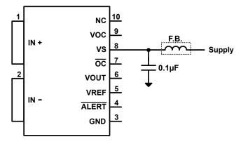
Figure 9-4. Power Supply Noise Filtering
