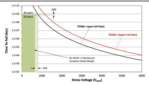
Figure 8-2. Insulation Lifetime
