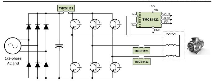
Figure 9-2. Inline Motor Phase Current Sensing
