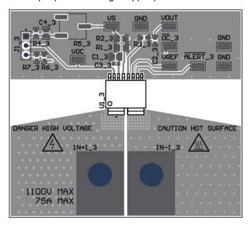
Figure 9-5. Recommended Board Layout
