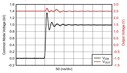
Figure 7-3. Common-Mode Transient Response
