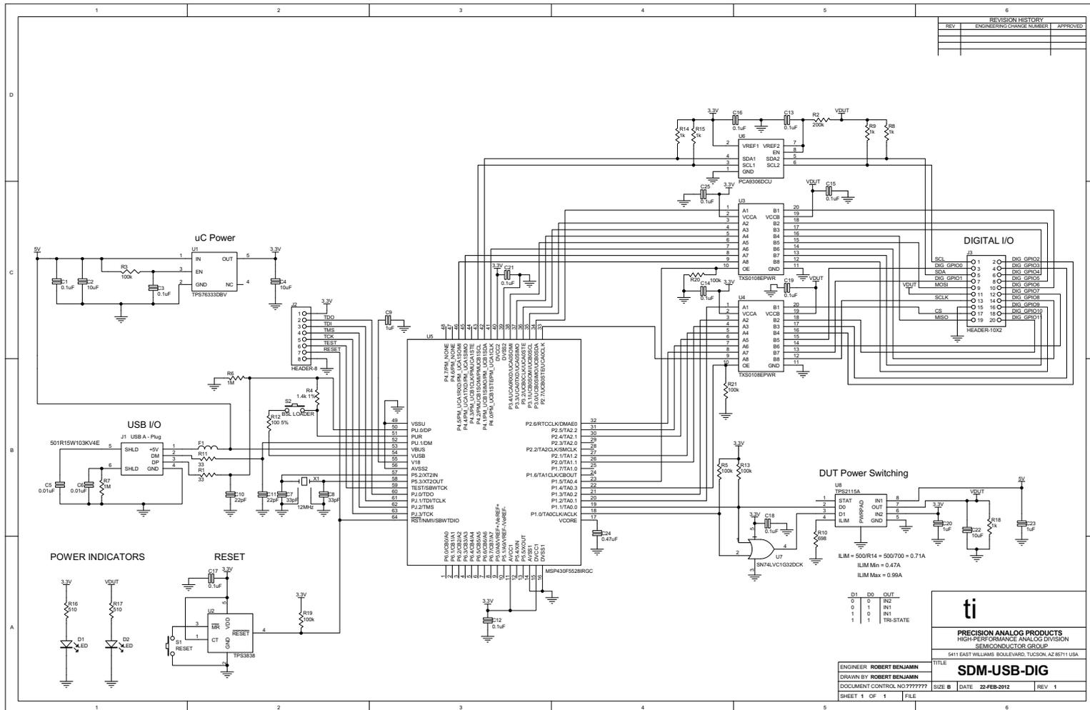
Figure 12. SDM-USB-DIG Schematic
