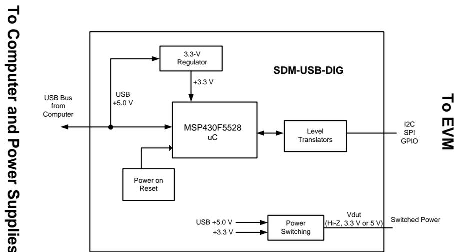
Figure 3. SDM-USB-DIG Platform Block Diagram
