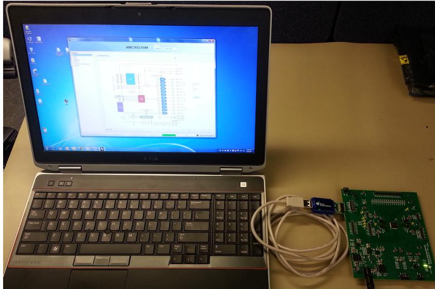
Figure 2. Typical Hardware Setup for the SDM-USB-DIG Platform
