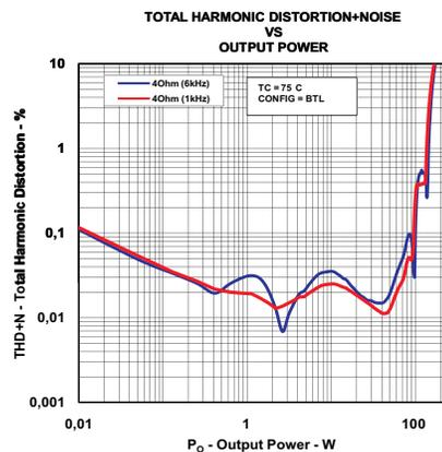
(1) Achievable output power levels are dependent on the thermal configuration of the target application. A high performance thermal interface material between the package exposed heatslug and the heat sink should be used to achieve high output power levels
