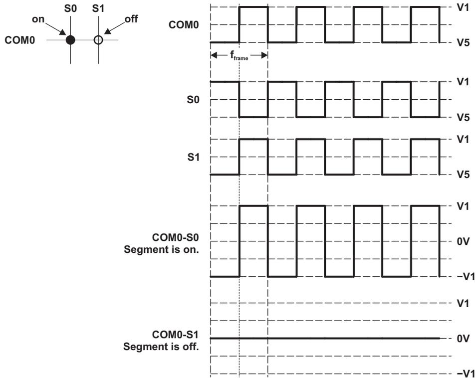
Figure 1-5. Example Static Waveforms
