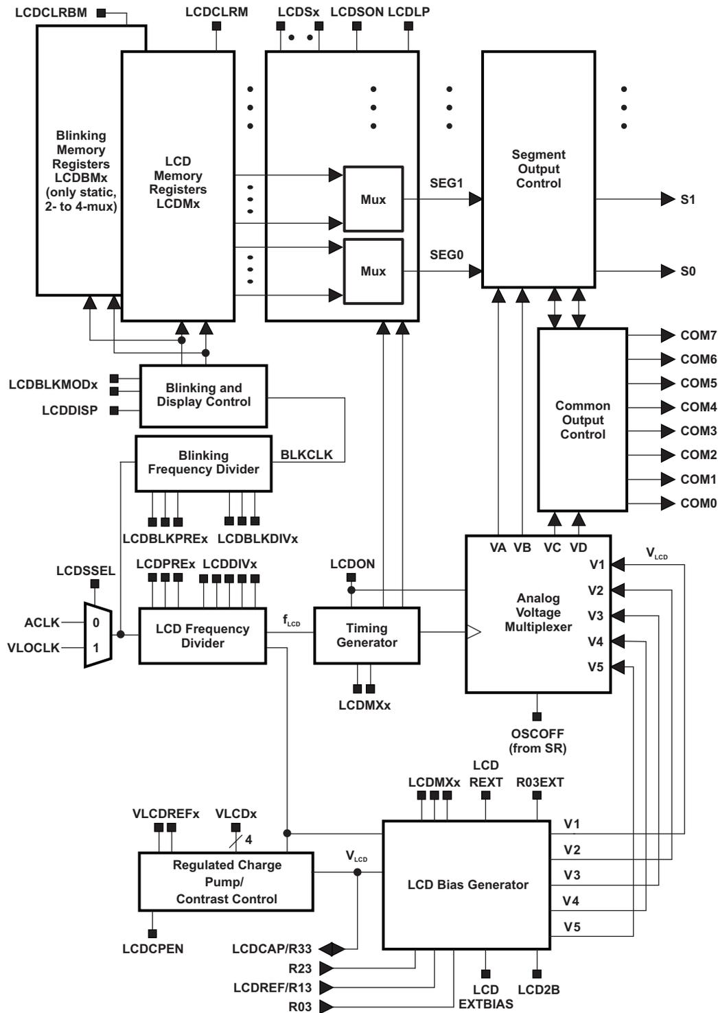
Figure 1-1. LCD Controller Block Diagram
