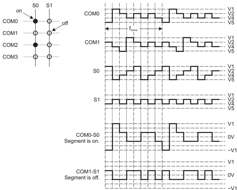
**Figure 1-8. Example 4-Mux Waveforms**
