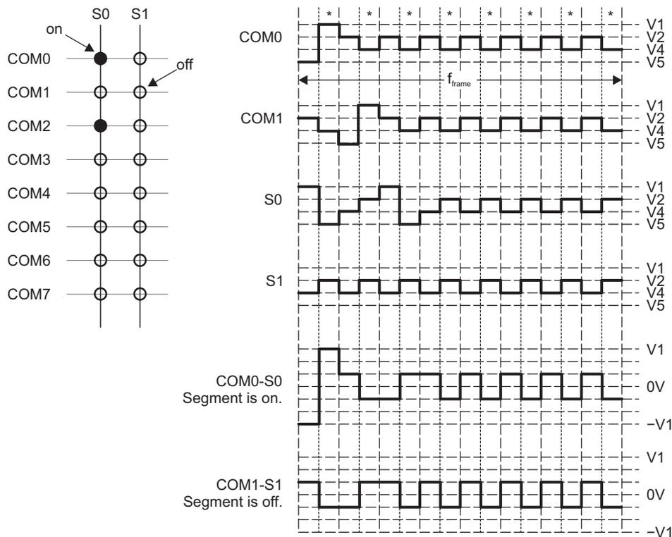
Figure 1-10. Example 8-Mux, 1/3 Bias Waveforms (LCDLP = 0)
