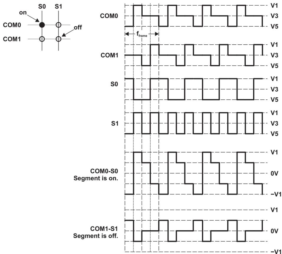
Figure 1-6. Example 2-Mux Waveforms
