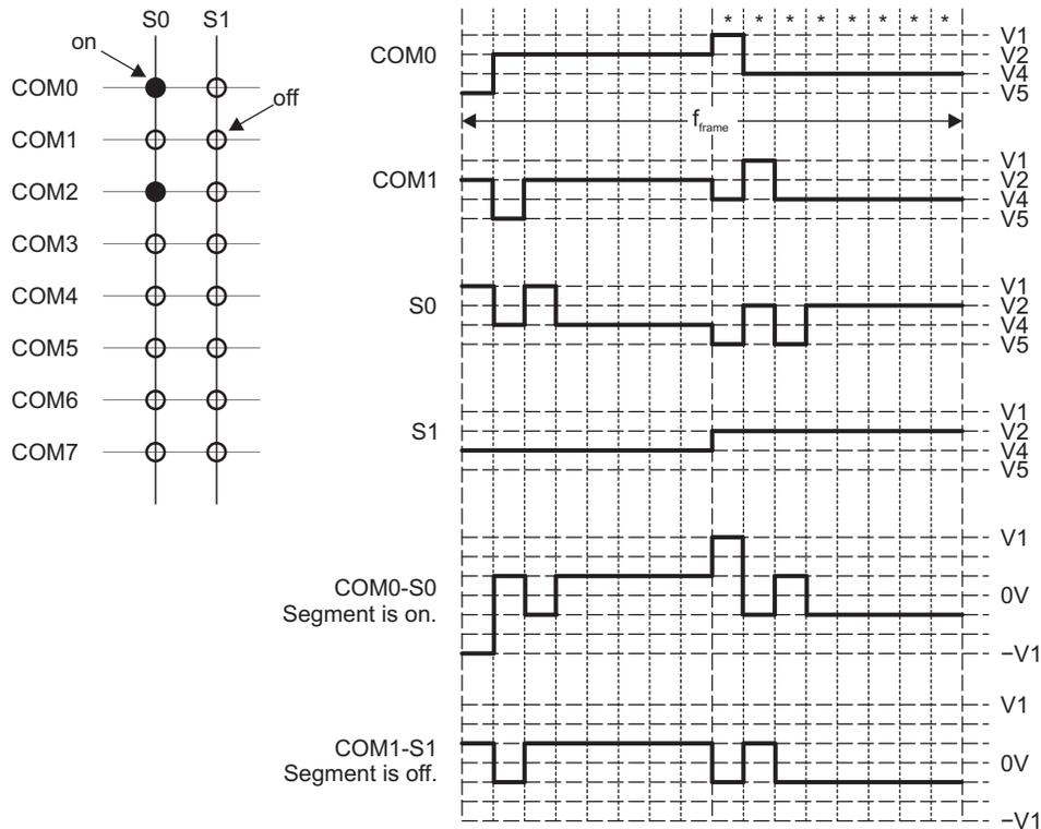
Figure 1-11. Example 8-Mux, 1/3 Bias Low-Power Waveforms (LCDLP = 1)
