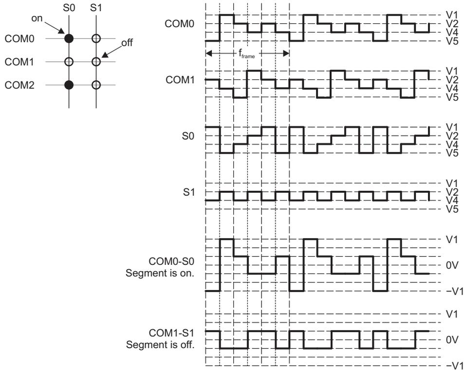
Figure 1-7. Example 3-Mux Waveforms
