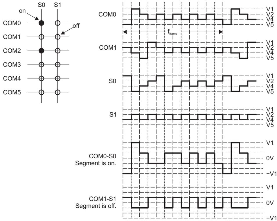
Figure 1-9. Example 6-Mux Waveforms
