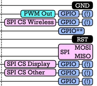
Below are the pins exposed @ the BoosterPack connector.
