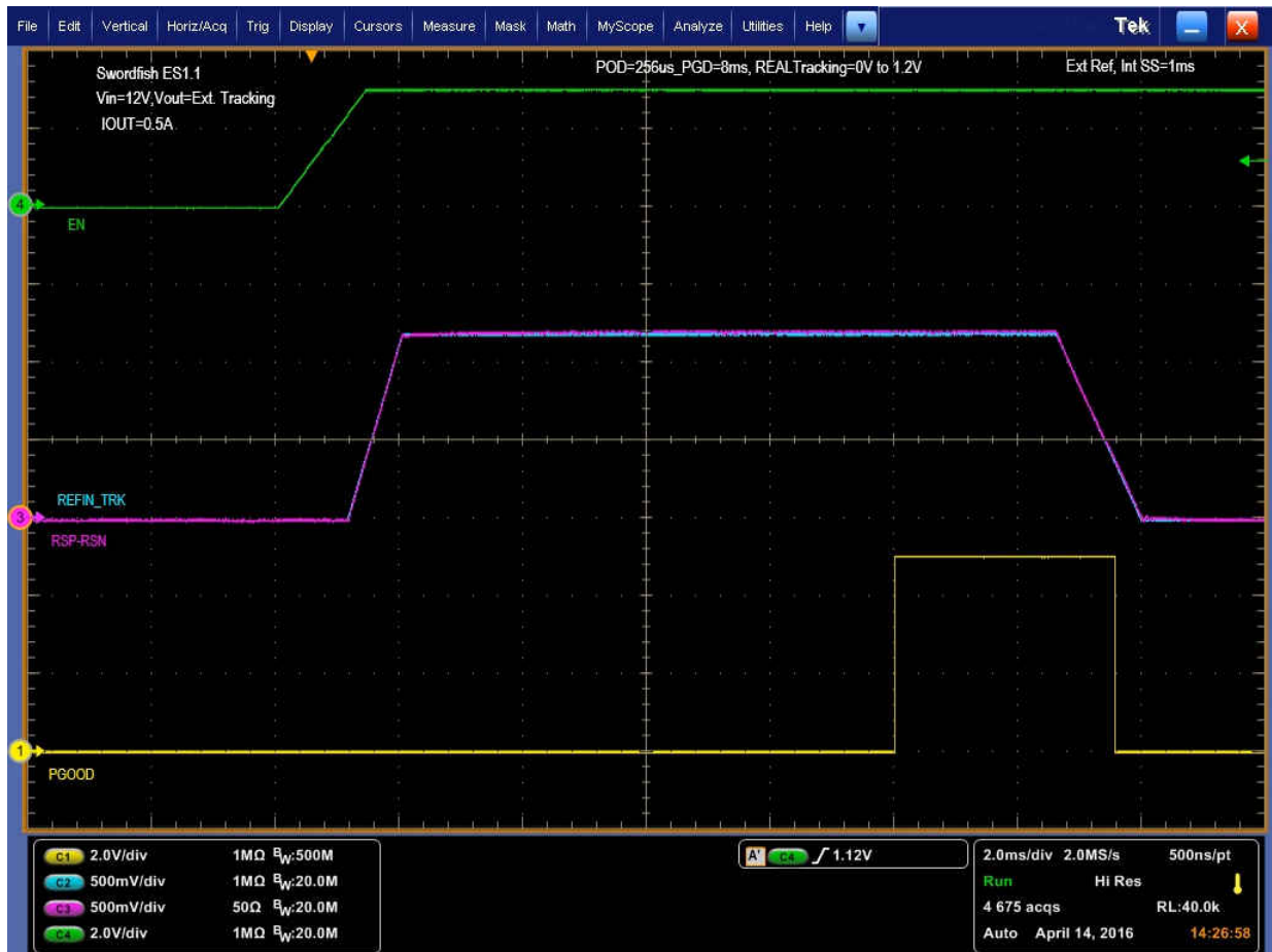
Figure 9-4. Real Tracking POD, 256 μs PGD 8 ms
