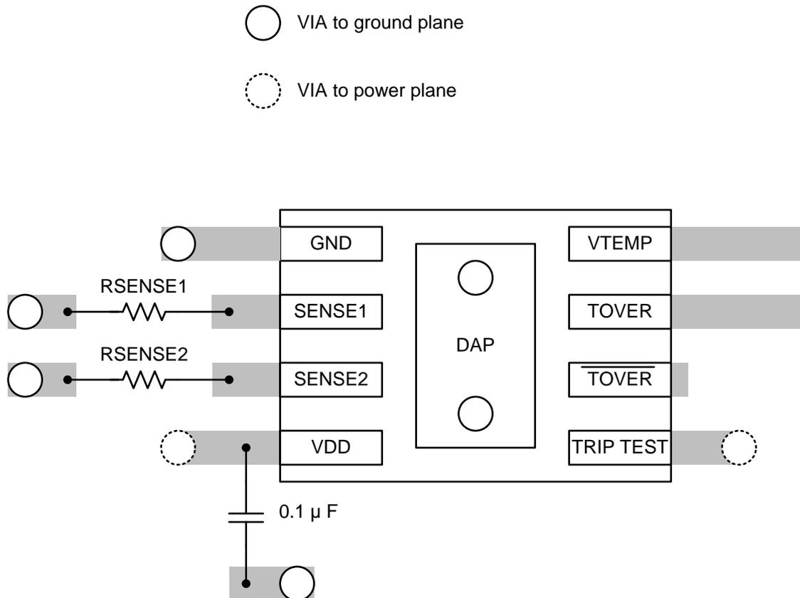
The best thermal conductivity to the junction of the LM57 is through the DAP. Make sure it is connected to the surface whose temperature that is being measured.
