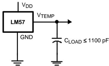
Figure 13. LM57 With No Isolation Resistor Required
