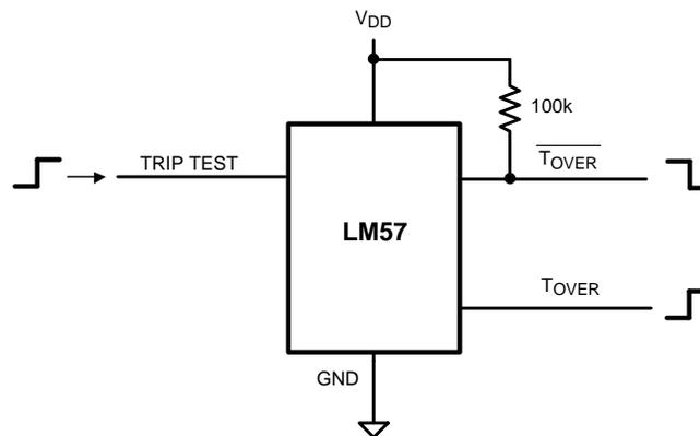
**Figure 17. Trip Test Digital Output Test Circuit**
