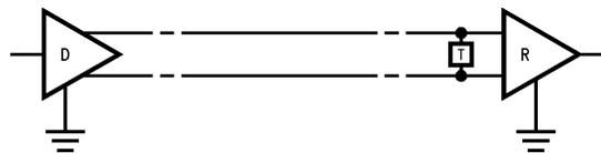
**Figure 7. Typical TIA/EIA-422-B Point-to-Point Application**
