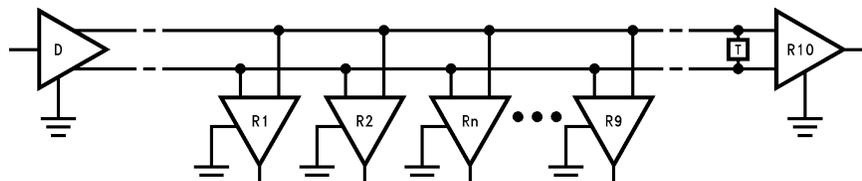
**Figure 8. Typical TIA/EIA-422-B Multidrop Application**
