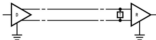
**Figure 14. MIL STD 188-114A Balanced, Type 2 Typical Application**
