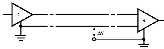
**Figure 12. MIL STD 188-114A Unbalanced Typical Application**
