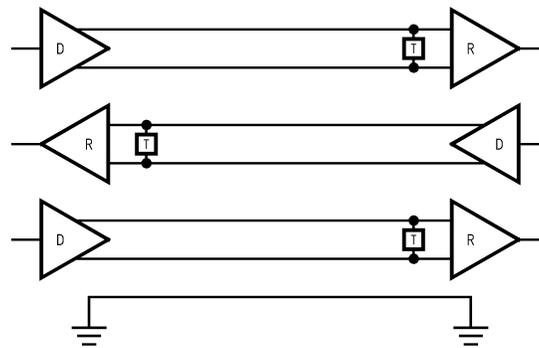
**Figure 2. Balanced Data Transmission- 3 Channel,
