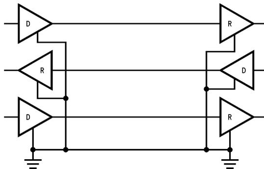
**Figure 1. Unbalanced Data Transmission- 3 Channel, 4 Line**
