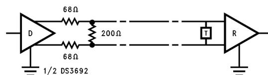
**Figure 13. MIL STD 188-114A Balanced, Type 1 Typical Application**
