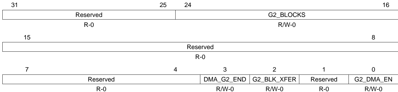
Figure 22-44. ADC Group2 DMA Control Register (ADG2DMACR) [offset = 54h]
