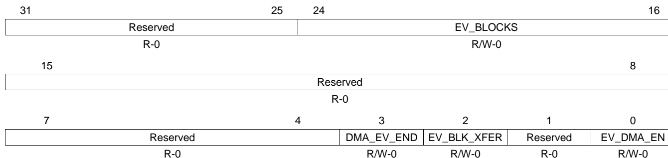
Figure 22-42. ADC Event Group DMA Control Register (ADEVDMACR) [offset = 4Ch]
