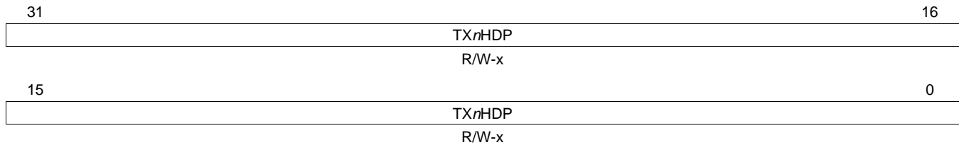
Figure 88. Transmit Channel n DMA Head Descriptor Pointer Register (TXnHDP)
