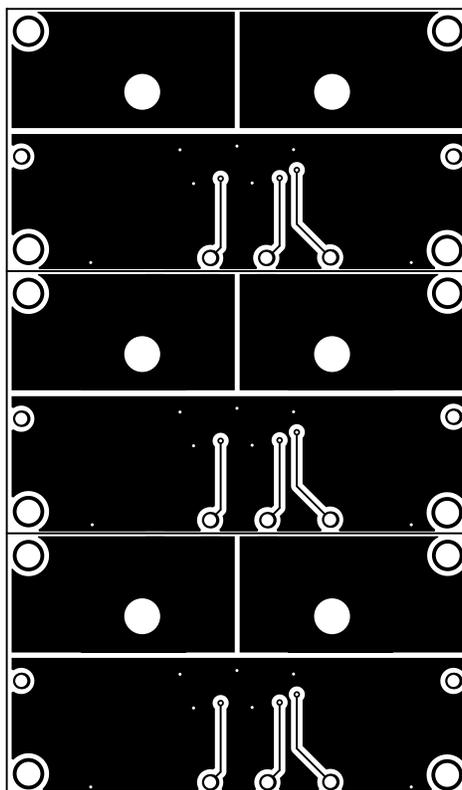
**Figure 5. PCB Bottom Layer**
