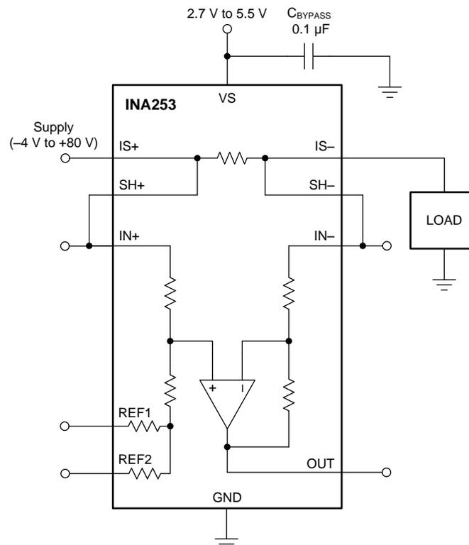
NOTE: This single block diagram is functionally equivalent for all EVM breakout boards.
