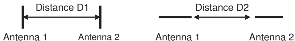
Figure D-1. Distance Between Antennas (Top View)
