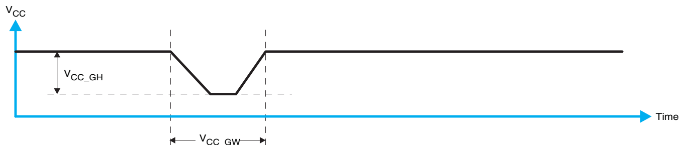
Figure 34. Glitch Width And Glitch Height
