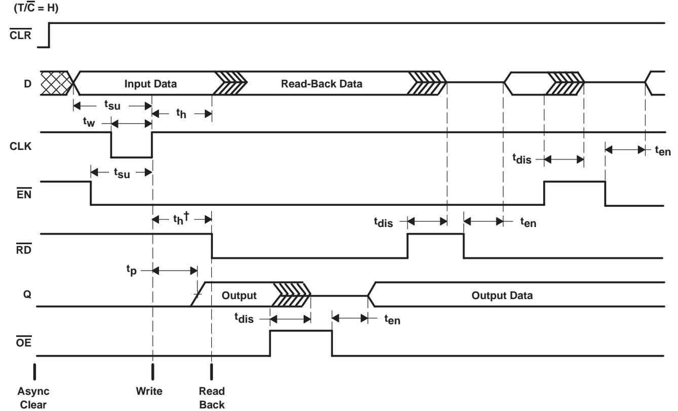
$^\dagger$  This hold time ensures that the read-back circuit will not create a conflict on the input data bus.
