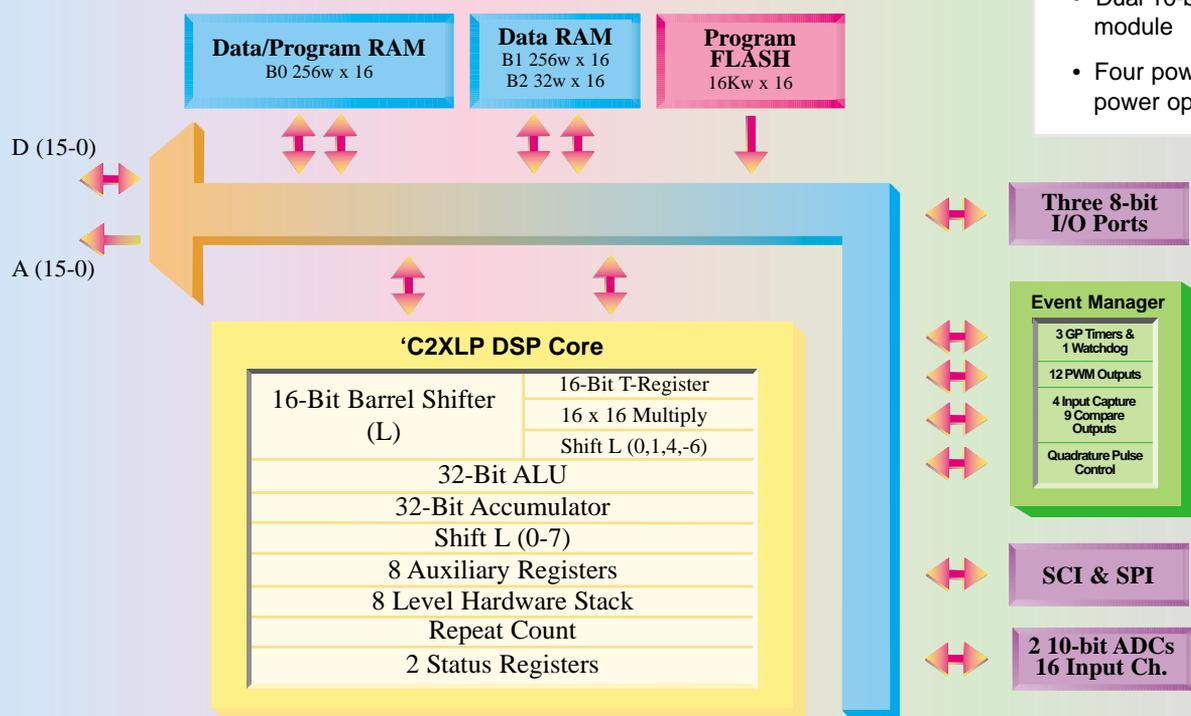
Texas Instruments Digital Signal Processor (DSP) controllers are revolutionizing today's motor control applications in appliances, HVAC, industrial drives, automotive and consumer electronics. The SMJ320F240 DSP has brought the performance and flexibility of the TI family of DSP motor controllers to the military and industrial markets.
