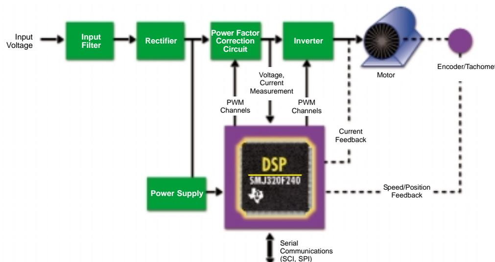
With a high level of peripheral integration and powerful computational abilities, the SMJ320F240 becomes the center of many different control applications.
