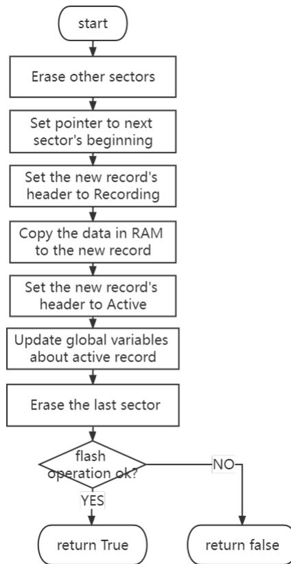
**Figure 3-8. Software Flow of EEPROM\_TypeA\_repairFormat**
