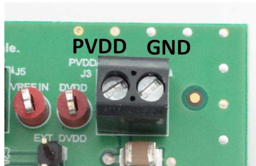
Figure 3. PVDD/AVDD, and DVDD Supply Connections
