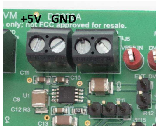
Figure 5. Onboard Reference Supply Connections
