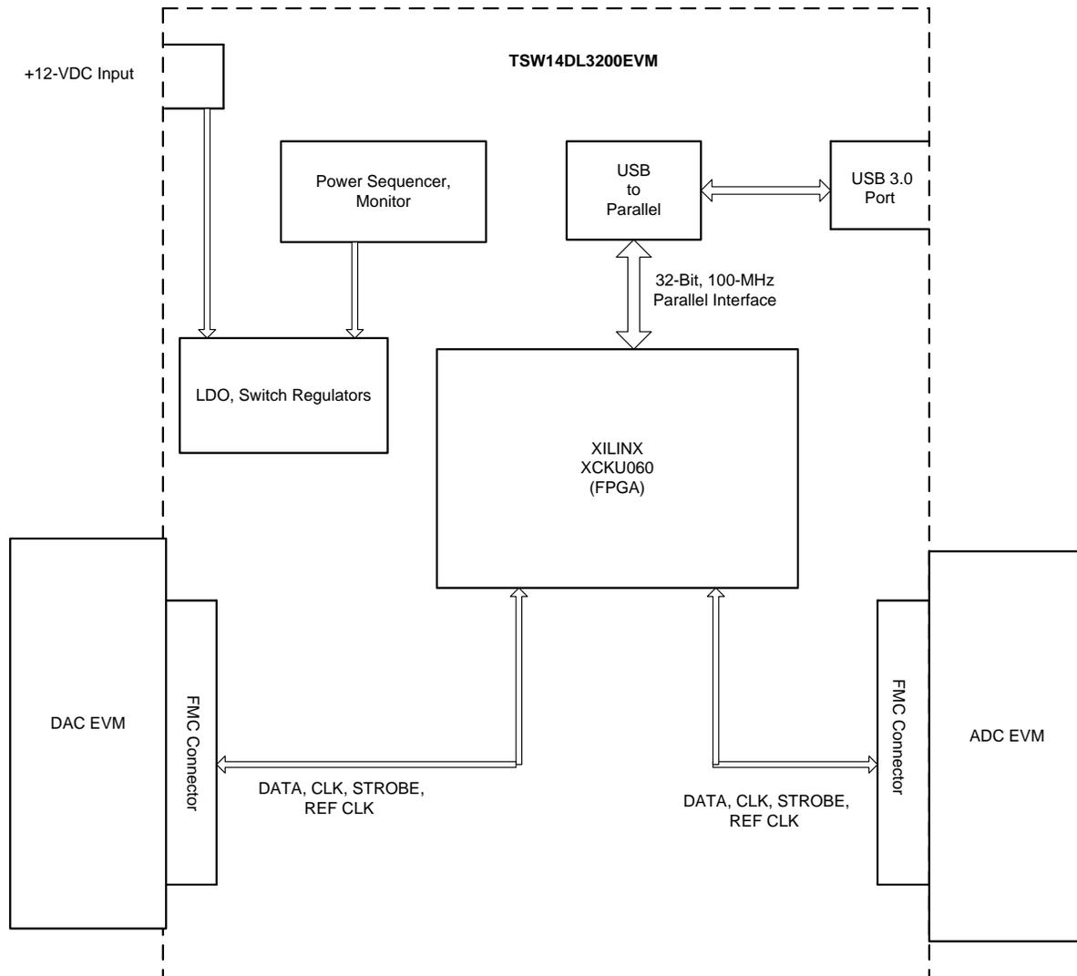
Figure 2. TSW14DL3200EVM Block Diagram
