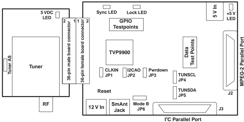
Figure 1. TVP9900EVM Block Diagram
