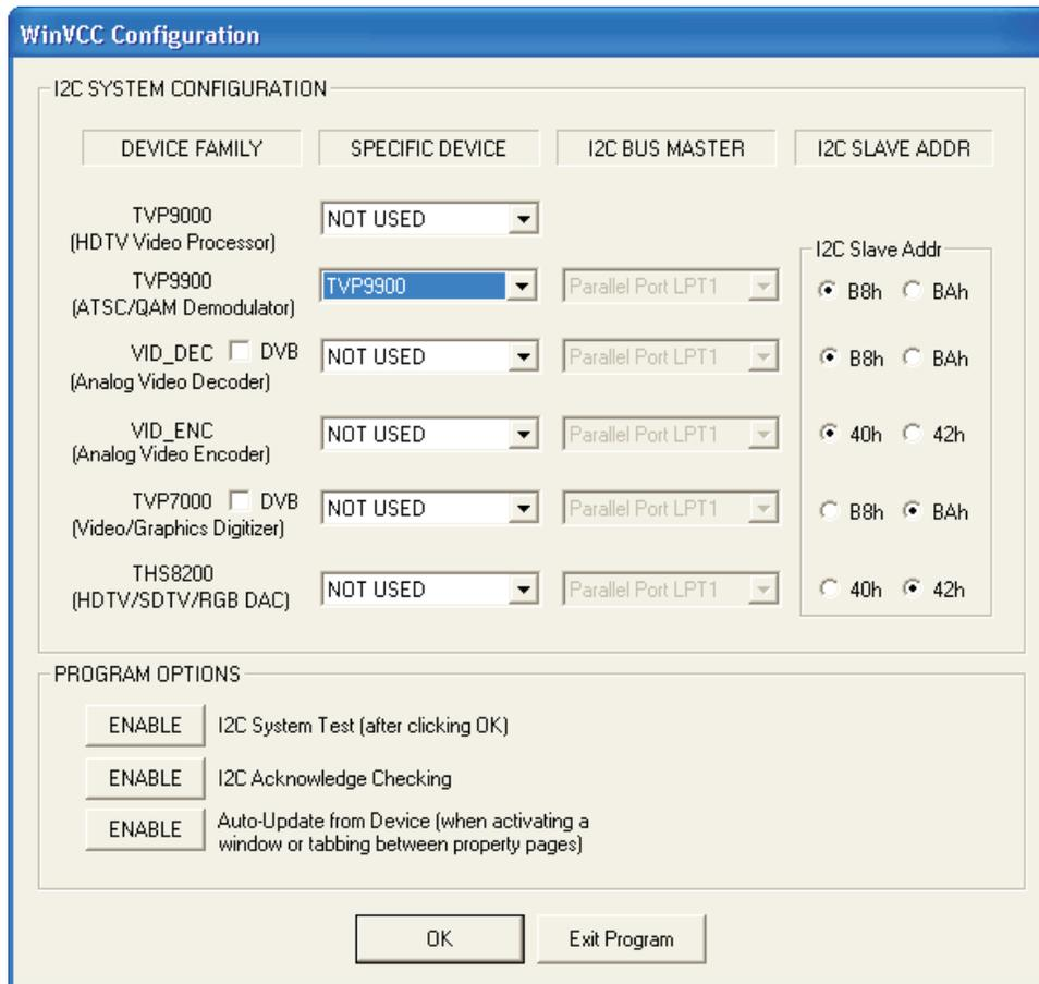
**Figure 3. WinVCC – I<sup>2</sup>C Configuration Screen**
