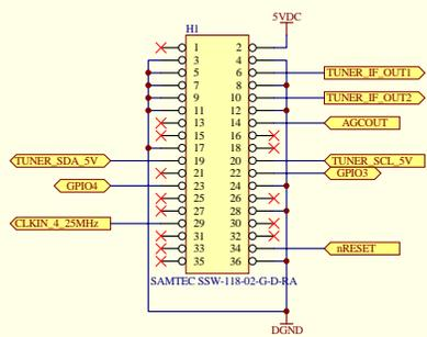
**NOTE:** Layout must support vertical or horizontal mount for tuner board
