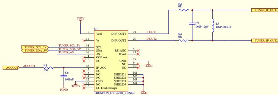
Uses Thomson DTT76801 with integrated DC to DC converter
