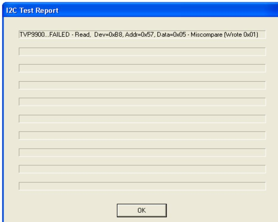
Figure 11. I<sup>2</sup>C System Failure
