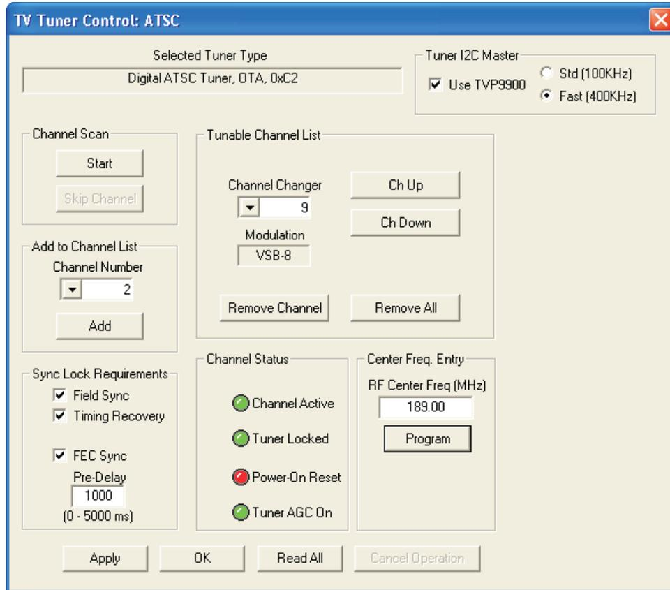
**Figure 7. TV Tuner Control for ATSC**
