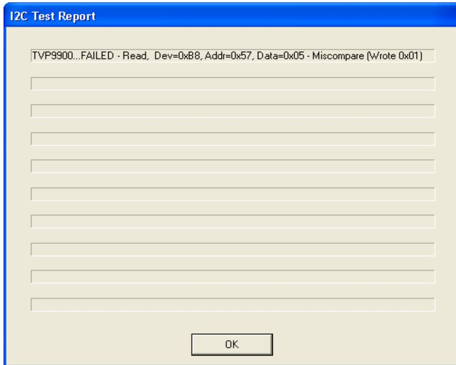
Figure 21. I<sup>2</sup>C System Failure Dialog Box
