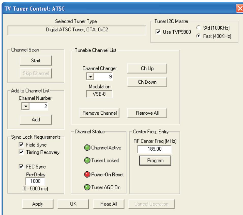
**Figure 20. TV Tuner Control for ATSC**
