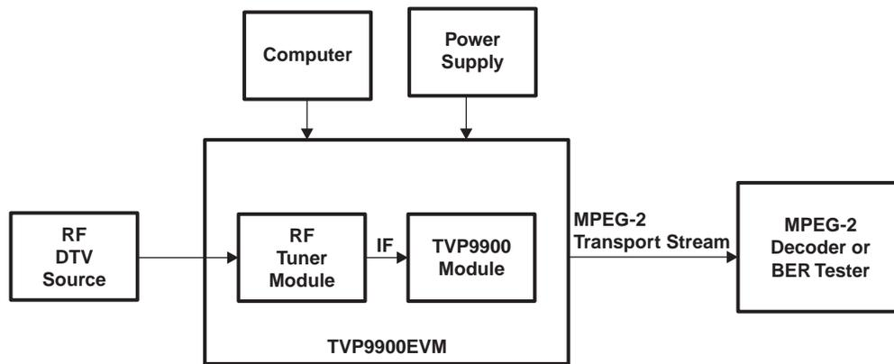
Figure 2. TVP9900EVM System-Level Block Diagram
