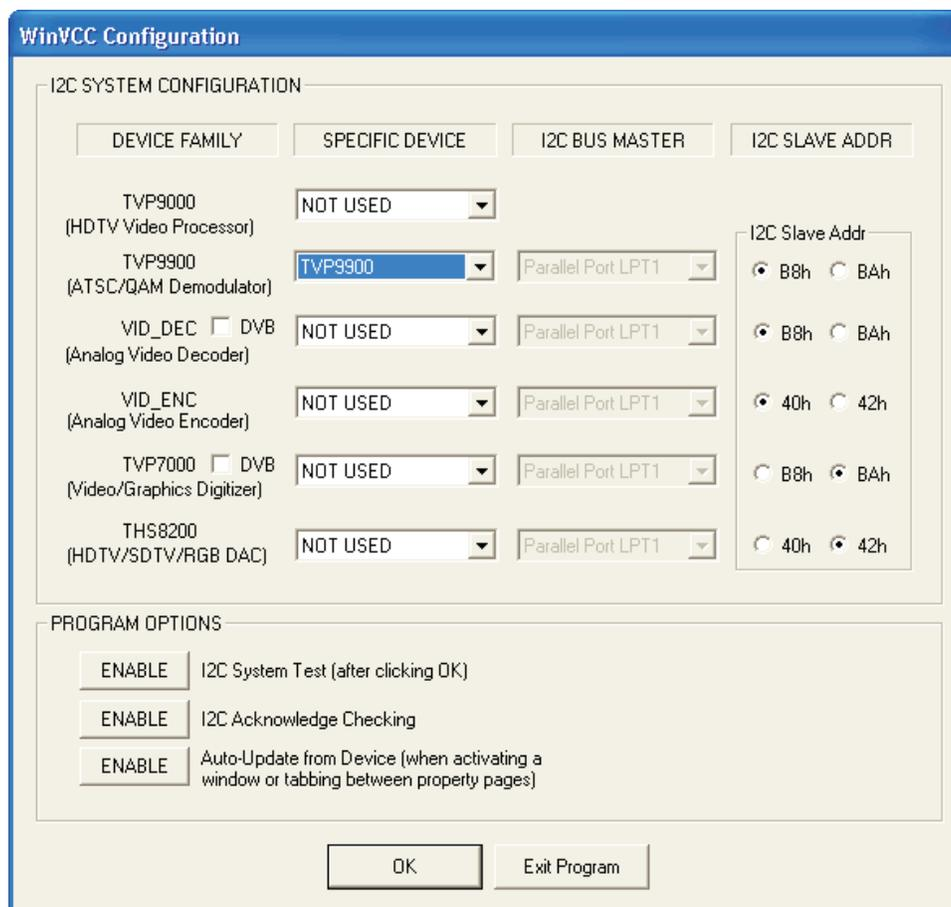
**Figure 10. WinVCC I<sup>2</sup>C Address Configuration**
