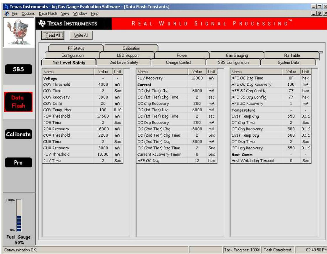
Figure 9. Data Flash Screen, 1st Level Safety Class
