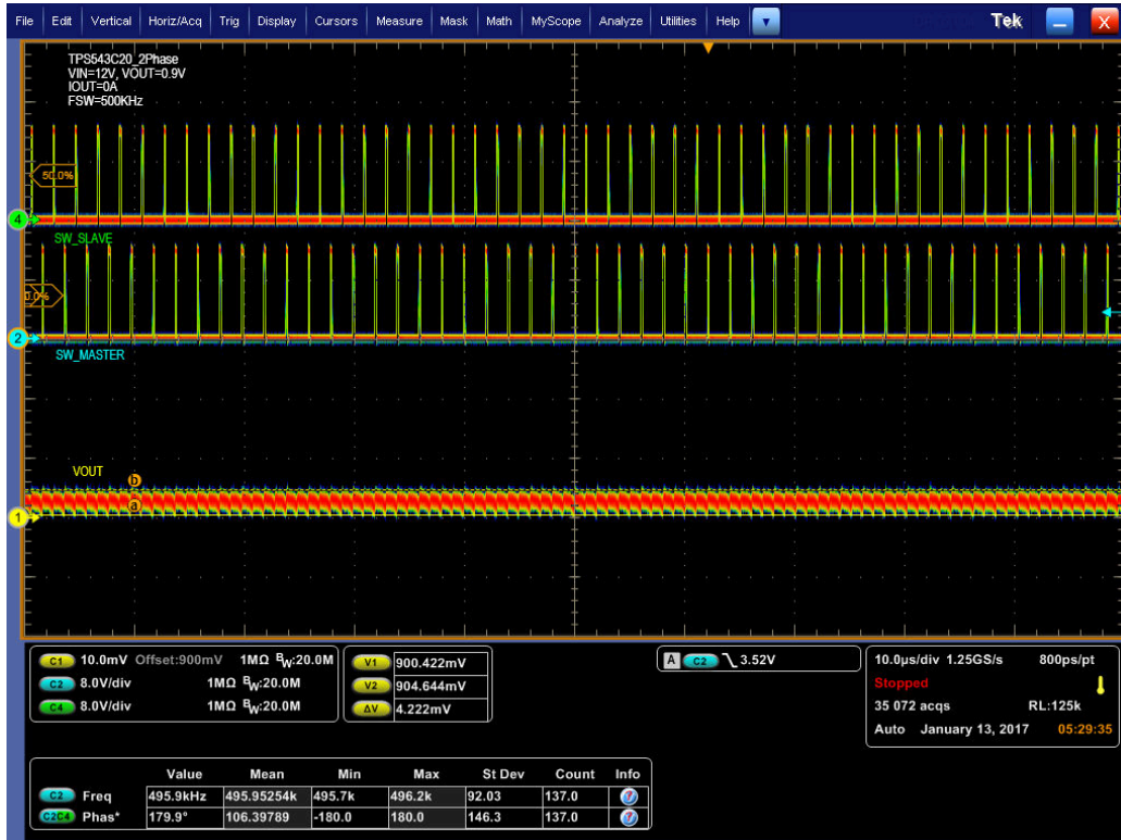
Figure 9-8. Output Ripple and SW Node of 0.9-V Output at 12 V IN , 0-A Output
