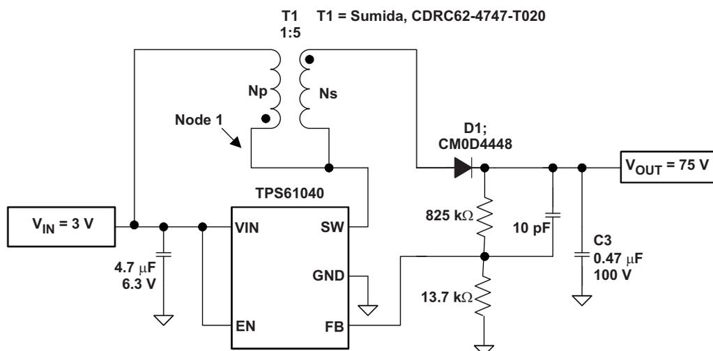
By substituting the inductor with a 1-to-5 transformer, the TPS61040 can deliver output voltages over 75 V. In this configuration, the output voltage can be achieved at any voltage as long as  $V_{sw}$  is kept below 28 V. This design generates a 75-V output that can supply up to 6 mA, depending on the input voltage.
