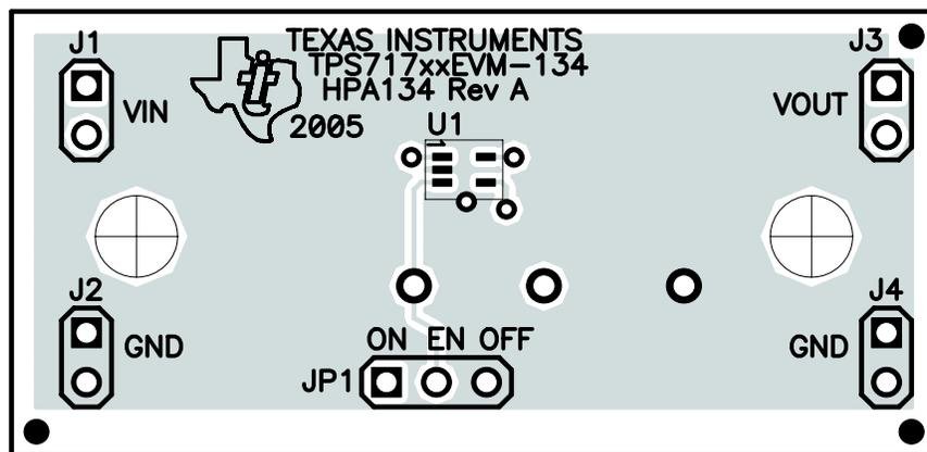
Figure 1. Assembly Layer
