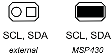
Figure 4. I 2 C Interface Jumper Settings
