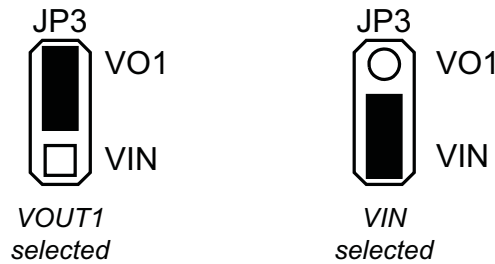
Figure 3. VINLR1 Jumper Setting
