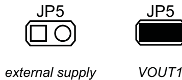
Figure 5. VSUP Jumper Setting
