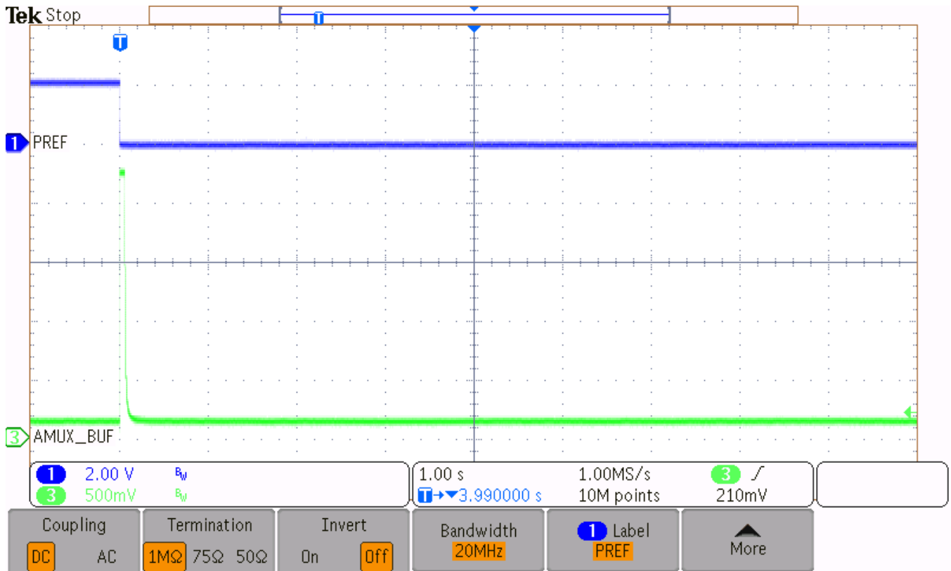
Figure 9. CO Connectivity Test without Sensor
