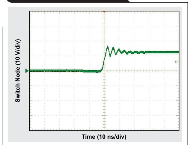
**Figure 5. Switch-node waveform with a boot resistor**
