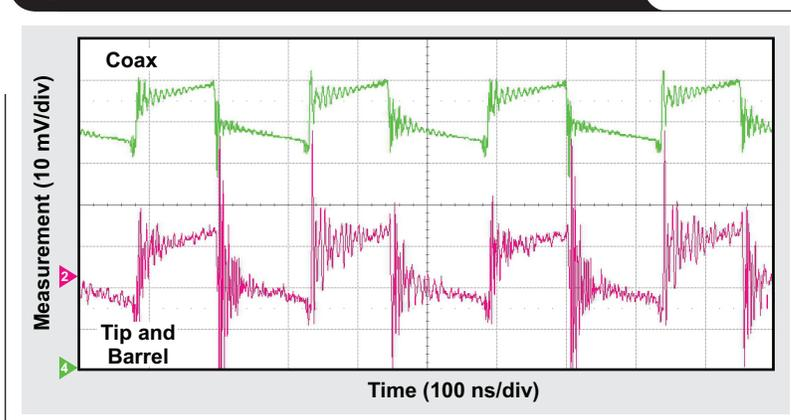
Figure 2. Original output ripple for the TPS54824
