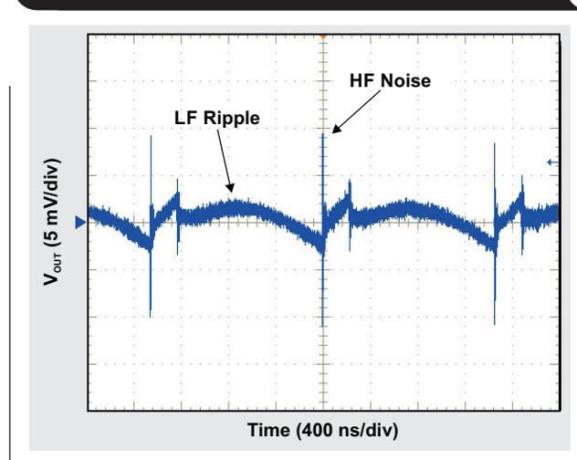
capacitance. The HF noise comes from the coupling of the switch node's high-frequency ringing through the parasitic capacitance of the inductor (the oscilloscope must have enough bandwidth to capture this, typically  $\geq 200$  MHz).
