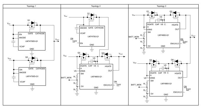
Figure 2. Typical ORing topologies using ideal diode controllers.
