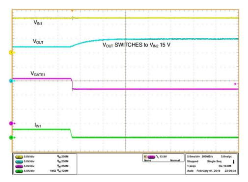
Figure 3. Supply switchover from VIN1 to VIN2.
