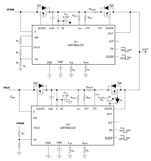
Figure 5. Typical priority power multiplexer application circuit using the LM74900-Q1.
