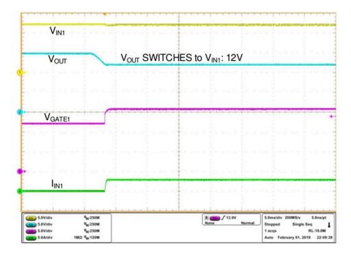
Figure 4. Supply switchover from VIN2 to VIN1.
