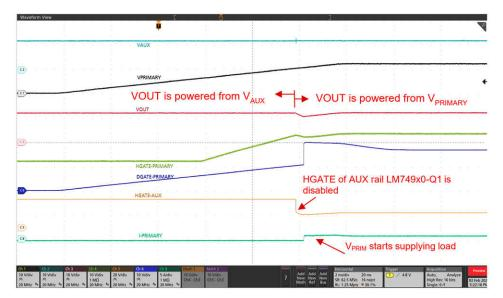
Figure 7. V<sub>AUX</sub> to V<sub>PRIM</sub> switchover in a power multiplexer application.
