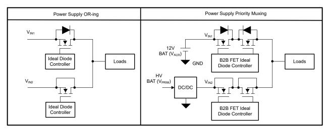
Figure 1. Typical use case of ORing and priority power multiplexer solution.
