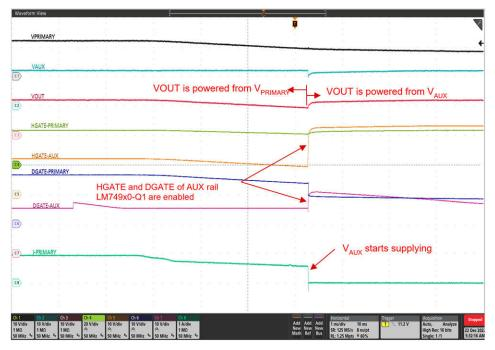
Figure 6. V<sub>PRIM</sub> to V<sub>AUX</sub> switchover in a power multiplexer application
