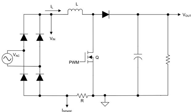
**Figure 1.** A common current-sensing method for PFC.
