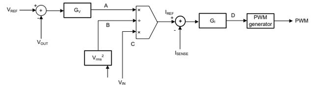
**Figure 2.** Traditional average current-mode control for PFC.
