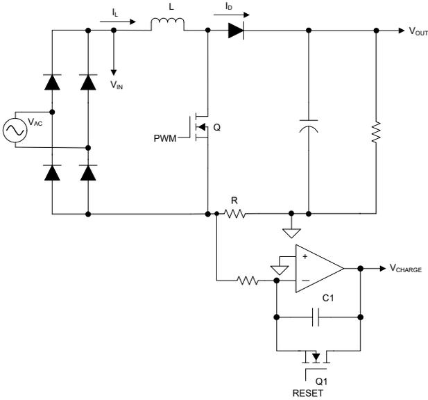
**Figure 3.** Using the current shunt and op amp to obtain an electric charge.
