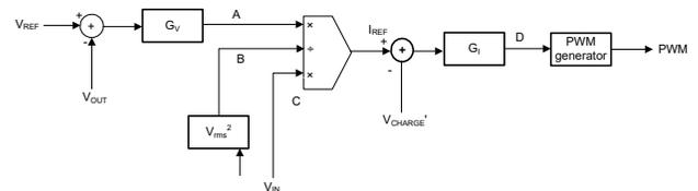
**Figure 7.** Charge-mode control law for PFC after eliminating RHPZ.
