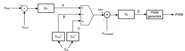
**Figure 6.** Charge-mode control law for PFC.
