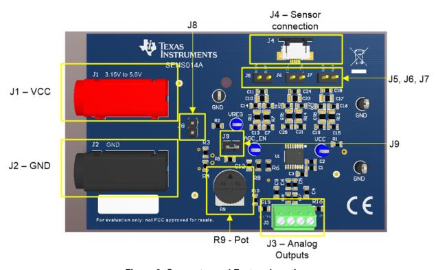
Figure 2. Connector and Feature Locations
