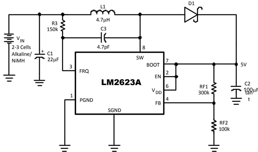
Figure 1. LM2623 Boost Converter for Digital Camera Motor
