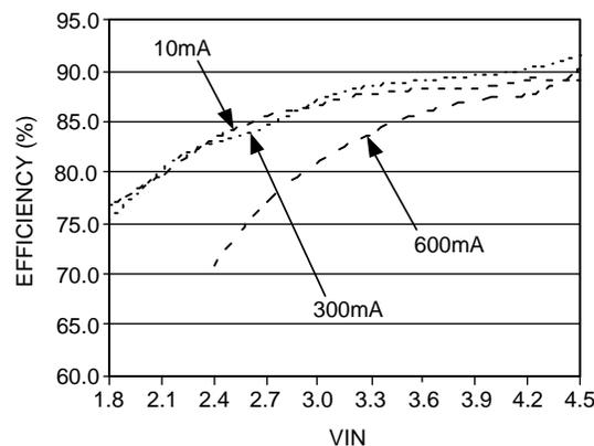
Figure 2. Efficiency for LM2623A Ratio Adaptive Circuit
