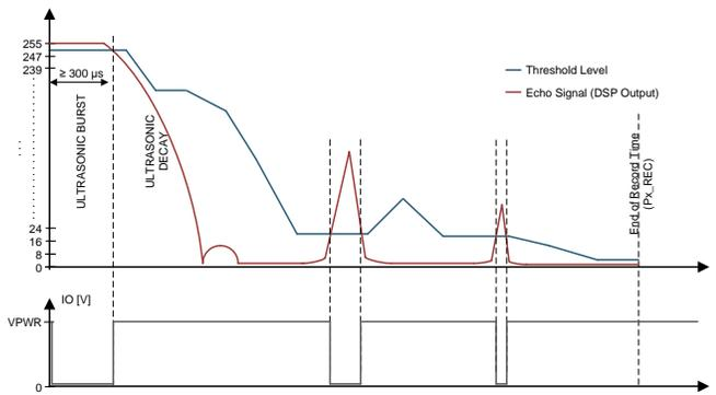
**Figure 5. Time Command Interface and Threshold Comparator**
