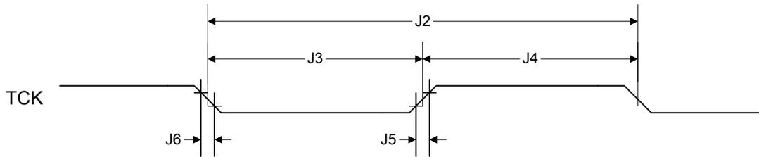
Figure 22-3. JTAG Test Access Port (TAP) Timing
