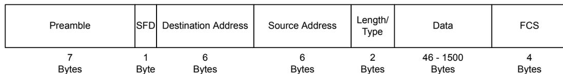
The seven fields of the frame are transmitted from left to right. The bits within the frame are transmitted from least to most significant bit.
