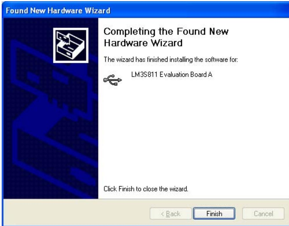
You have just installed the drivers for “LM3S811 Evaluation Board A.” The USB device built into the EVB is a composite USB device. After you click Finish, Windows automatically installs a driver for the “Luminary Micro ICDI Board B” part of the composite USB device. Follow the same instructions as above to install the drivers for this device.
