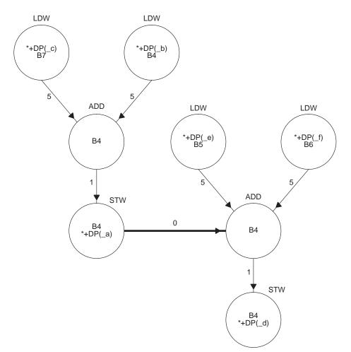
The circles are called nodes, and the arrows connecting the circles are called edges. There is one node for each instruction, and one edge for each dependence. Since instructions can have multiple dependences as both input and output, nodes in the graph can have multiple edges leading in and out.
