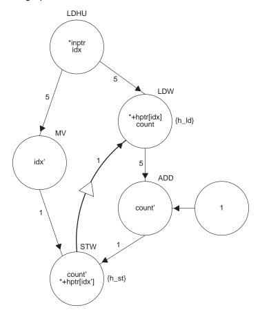
Note the flow dependence memory edge, carried by the loop, from the STW to the LDW. Now the assembly optimizer generates a 7 cycle loop. Much slower, but it works.
