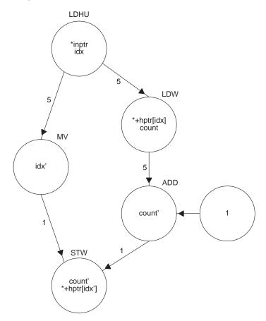
Note the assembly optimizer splits the lifetime of the idx register by adding the MV instruction; the new variable is shown as idx'. The lifetime of count is similarly split at the ADD instruction.
