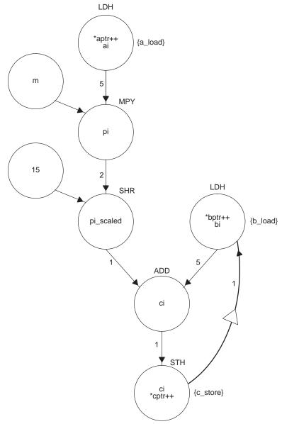
Now, instead of the anti-dependence memory edge, there is a flow dependence memory edge from c\_store to b\_load. Note this dependence is carried by the loop. Now the assembly optimizer generates a 7 cycle loop.
