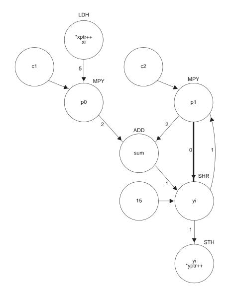
Consider the instructions which reference yi. Note the flow dependence, carried to the next iteration by the loop, on yi from the SHR to MPY, because the SHR writes a value to yi which MPY reads. Also note the anti-dependence, not carried by the loop, on yi from the MPY to the SHR, because the MPY must read yi before SHR writes to it. Note how the two dependences are in opposite directions.
