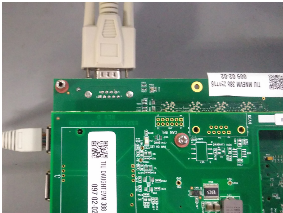
Figure 7. Serial Cable Connected to EVM
