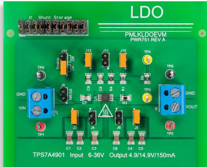
Figure 6. TPS7A4901 LDO board: jumpers set-up for Test#1
