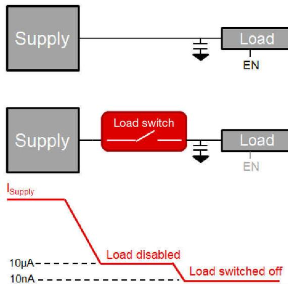
**Figure 2. Adding a Low-leakage Load Switch Reduces Shutdown Current**
