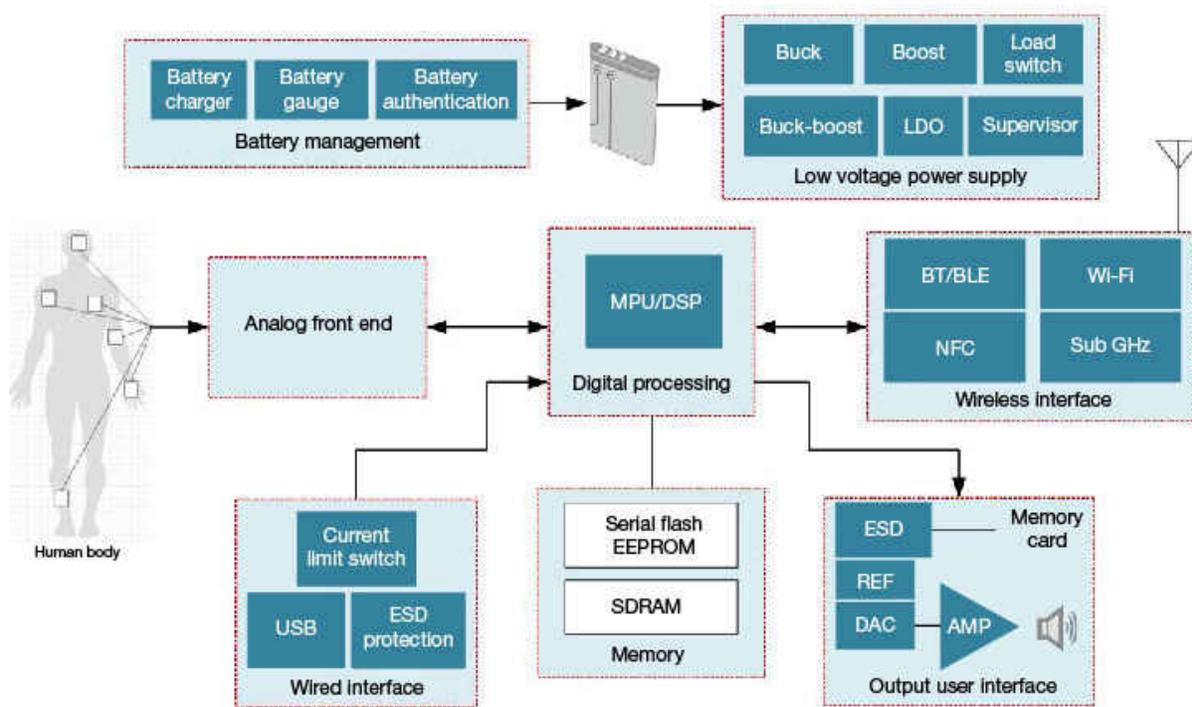
Figure 1. High-level Block Diagram of a [wearable patient monitor](#)
