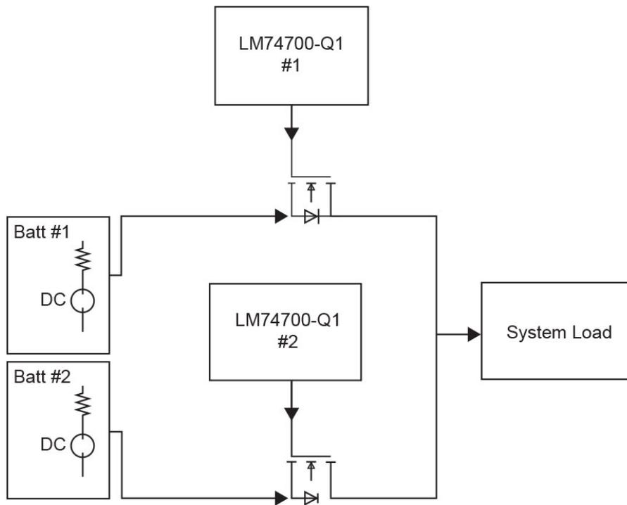
**Figure 1. A system block diagram with multiple batteries**
