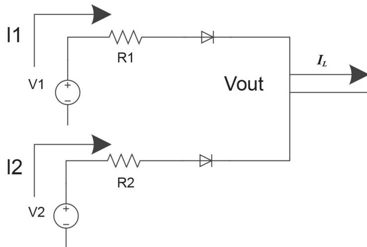
**Figure 3. Schematic of an equivalent resistance in the discharge path**
