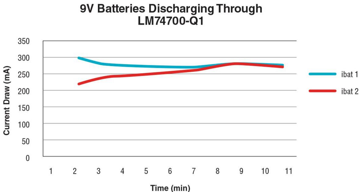
**Figure 2. Current draw from two 9-V batteries**
