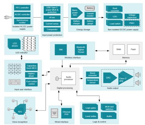
Figure 1. Smart Speaker Block Diagram
