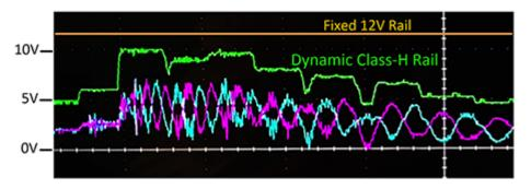
Figure 2. A Dynamic Supply Rail Saves Significant Power over a Fixed Rail
