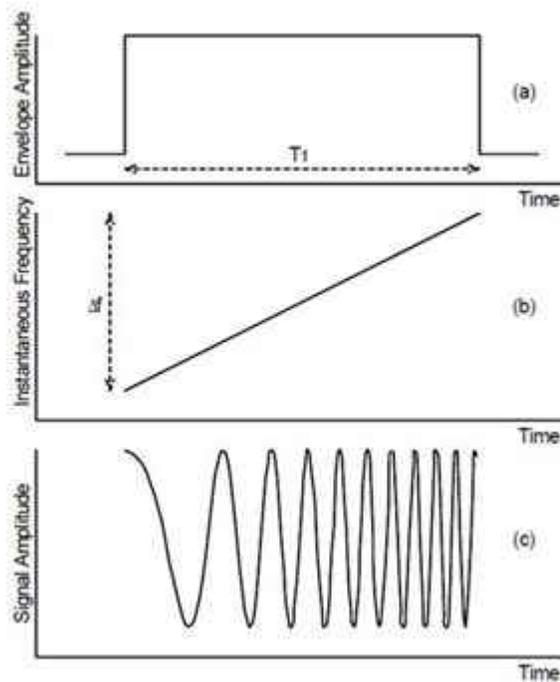
**Figure 3. Waveform of a Frequency-modulated (FM) Chirp**
