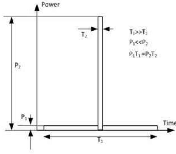
**Figure 2. Concept of Pulse Compression**
