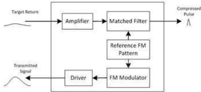
**Figure 4. A Simplified Block Diagram of an FM Chirp Sonar**
