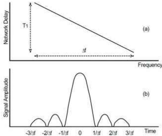
**Figure 5. Compressed Pulse after Matched Filtering**
