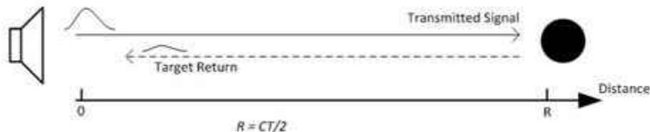
**Figure 1. Sonar Used in Target-range Measurement**
