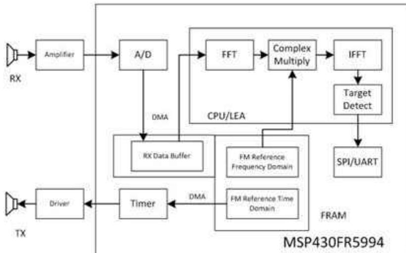
**Figure 7. FM Chirp Sonar Implemented on TI's MSP430FR5994 MCU**
