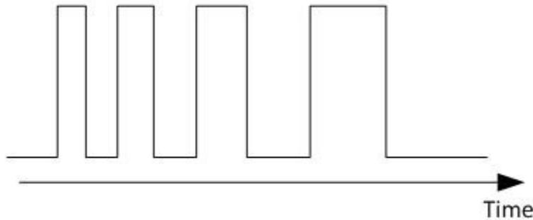
**Figure 8. Excitation Signal for the FM Chirp**
