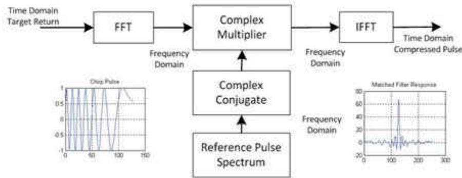
**Figure 6. Implementation of an FM Chirp Receiver**
