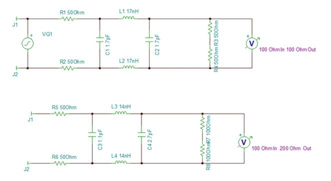
Figure 3. Filters with Different Impedance Ratios
