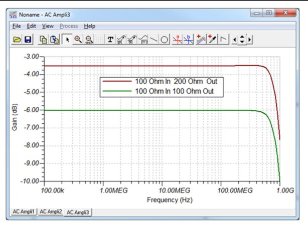
Figure 4. Filter Responses for Different Impedance Ratios
