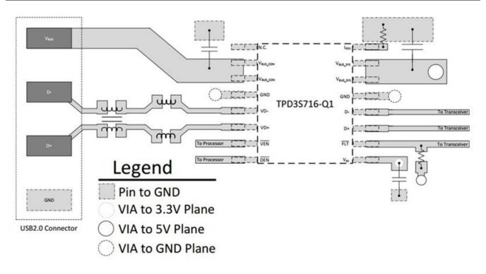
Figure 3. Typical Layout Example for the TPD3S716-Q1
