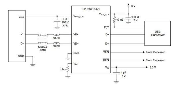
Figure 1. Typical Application Configuration for the TPD3S716-Q1
