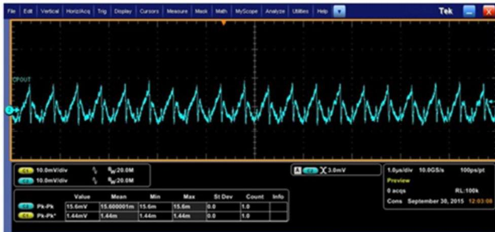
Figure 1. Charge-pump Output Characteristic
