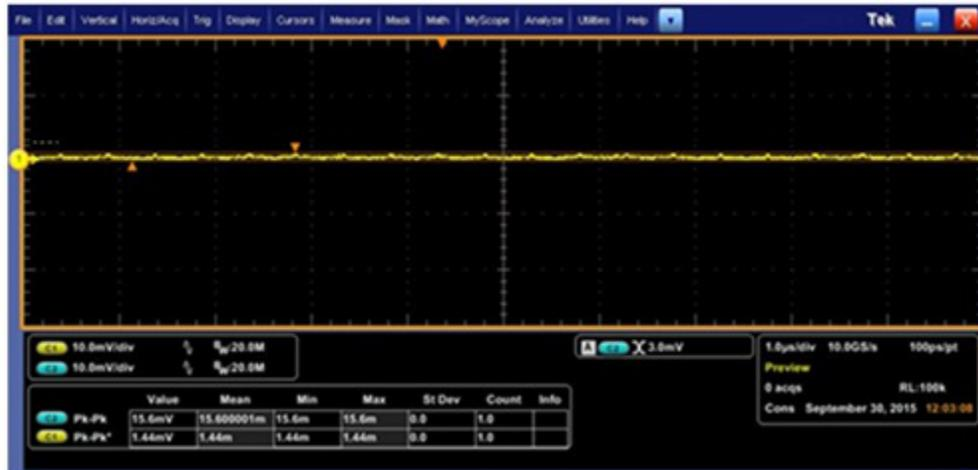
**Figure 2. Cleaned LDO Output**
